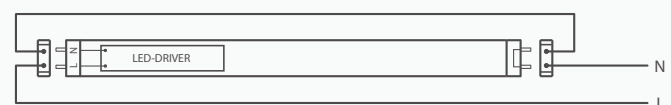
The G3 LED tubes can be inserted either way in the end sockets.
